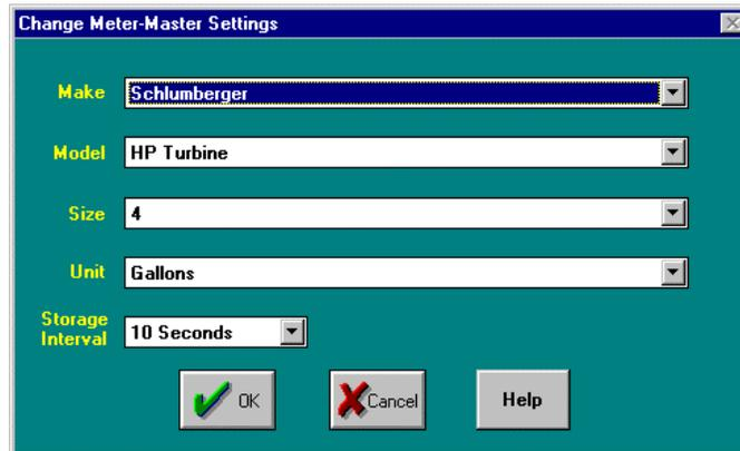
The Data Storage Interval is the only setting that directly affects the recording of data. A 10 second interval provides adequate resolution in most cases and 15 days of recording time (see box later in this section, “About The Data Storage Interval”).
