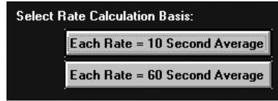
Generally, choose the 10 second average unless you are recording from a large, slow-pulsing meter (meter preceded by an asterisk in Appendix A), in which case a 60 second average is recommended. If the graph displays a spiking effect (large variance in flow rates during short time periods) when the flow rate appears relatively steady on the meter register's dial face, use the 60 second average.
