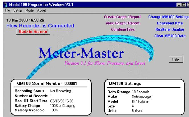
Batteries last approximately 3 months with a full charge. Whenever possible, connect the charger to the Meter-Master so that the batteries remain as fully charged as possible.
