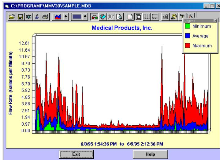
The Graph Screen generates, displays, prints, and saves graphs from a data file in a variety of styles. Each plotted vertical bar represents one Grid Interval, which can be viewed/edited on the Data Grid Screen before a graph is created. You may double-click anywhere on the colored portion of a graph, and a balloon will appear with data associated with the two (2) closest intervals.
