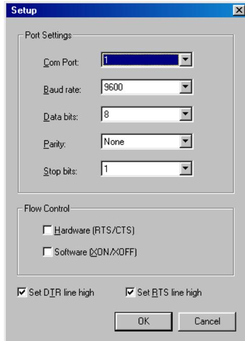
The Port Settings may be changed at any time by clicking the "Setup" menu bar option at the top of the Main Screen and choosing "Port" (the Meter-Master does not have to be connected). The default baud rate is 9600.
